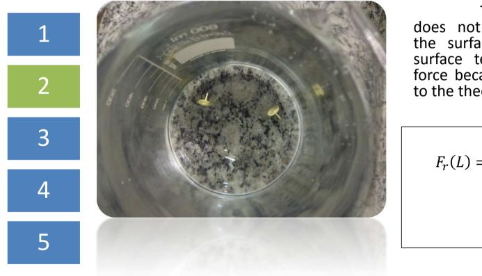
The phenomena does not occur, because the surfactant break the surface tension, and the force became 0, according to the theory.
