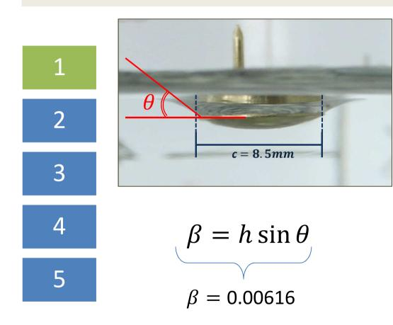
m = 0.0003kg  $\gamma_{water} = 0.0728 N/m$   $\theta = 38^{\circ}$ Temperature: 20°C Radius: 24.62 mm h: 0.00103 m
