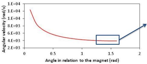
Angular velocity approximately constant near the normal line to the magnet.
