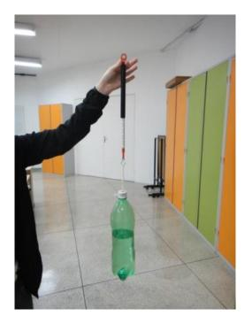
The dynamometer was calibrated with PET bottle full of water, with exact 1 kg, measured with a scale of precision of 0.1 g. The maximum mark of the dynamometer is 10N.
