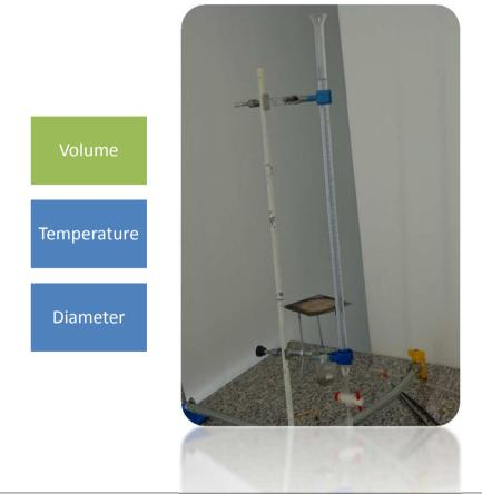
Tube diameter: 15 mm Syringe: 20 ml Fluid: Glycerin Temperature: 20°C
