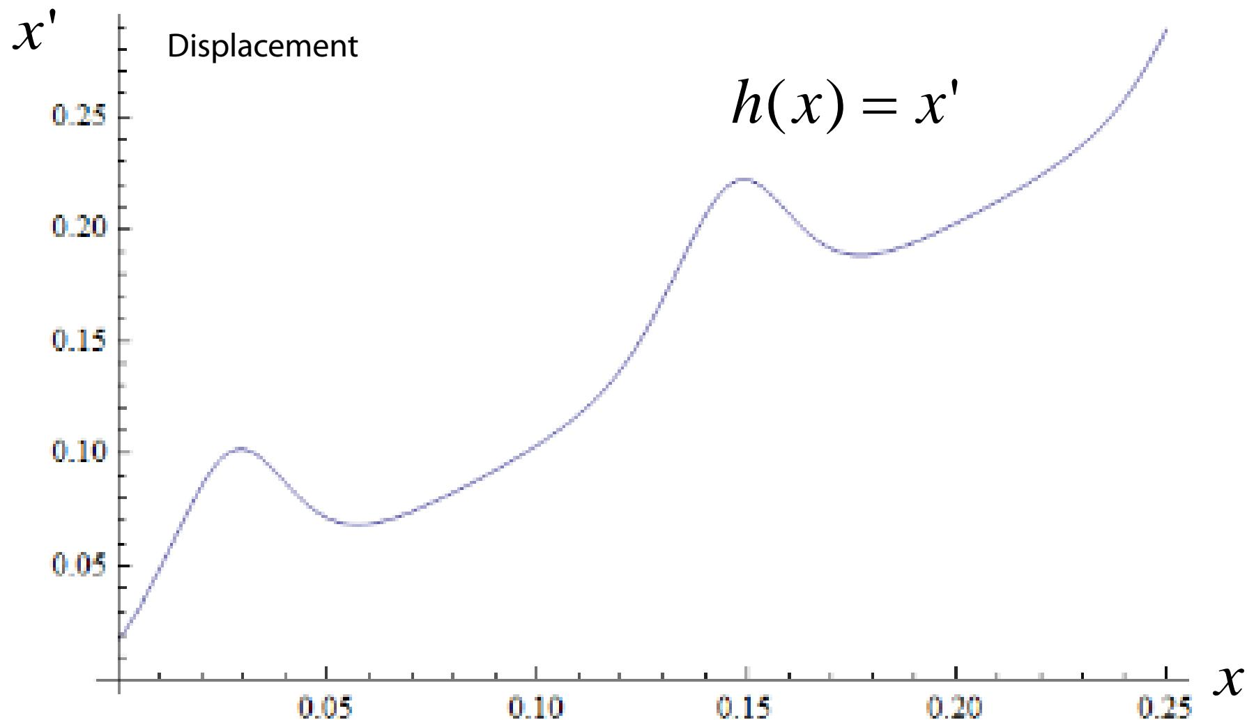
$$f[x_1] := x + \left( h + \frac{a}{2} + \frac{a}{2} * \cos[\pi * \frac{x}{1}] \right) \left( \tan[\pi / 4 - \text{ArcTan}[-a * \frac{\pi}{2 * 1} * \sin[\pi * \frac{x}{1}]]] - \text{ArcSin}[\frac{n1}{n2} * \sin[\pi / 4 - \text{ArcTan}[-a * \frac{\pi}{2 * 1} * \sin[\pi * \frac{x}{1}]]]] \right)$$
