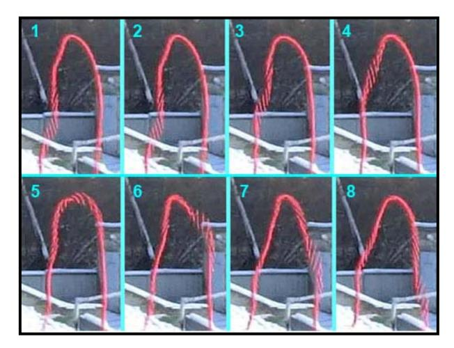
Time between frames = 1/240 s. Velocity of beads = 7 m/s. Velocity of the wave = 14 m/s.
