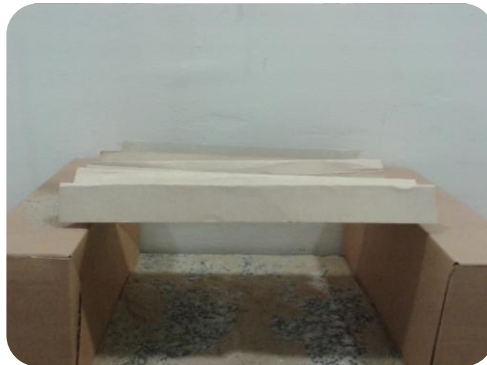
Corrugated fiberboard ( 237\text{g/m}^2 )
