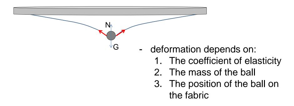
Shape can't be calculated analytically because of big deformations  $\rightarrow$  it was determined experimentally
