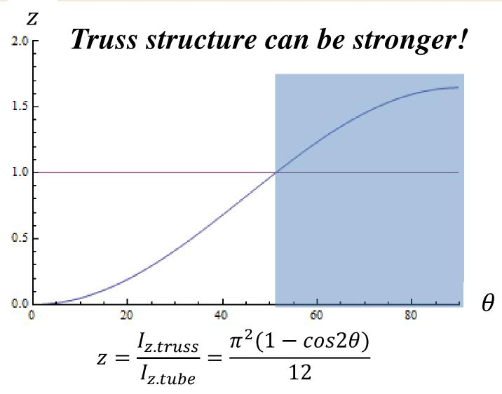
\*  $\theta$ : contact angle in truss structure
