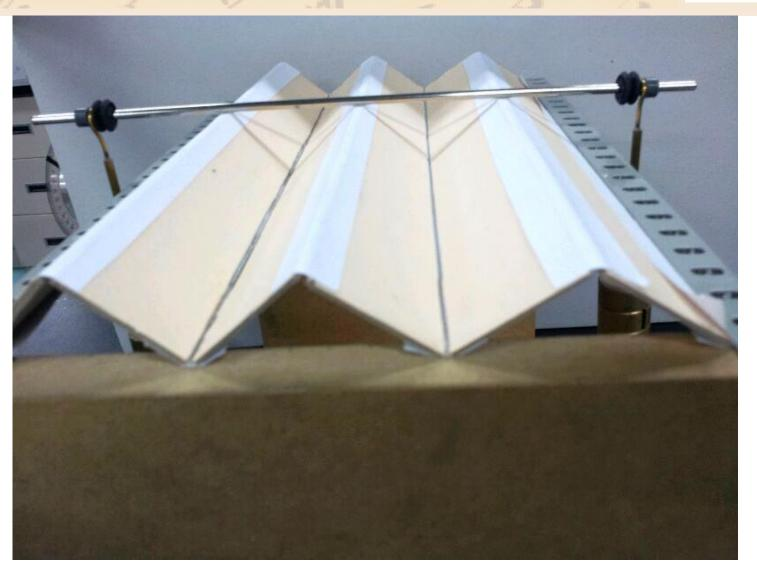
Thick paper bridge → eliminate necking and bending
