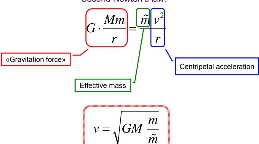
Velocity of the ball on a circular orbit is independent of the radius.
