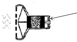
Without hole – overpressure inside the microphone – diaphragm bulks out
