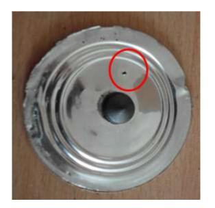
Hole in diaphragm used for pressure equalisation
