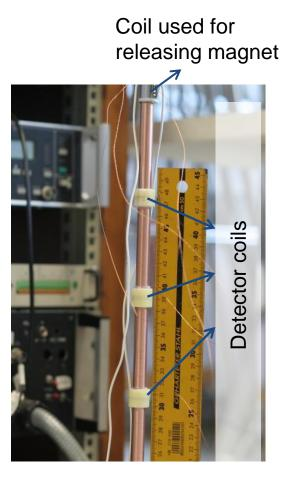
Velocity measurement – coils detect passing magnet due to induction:
