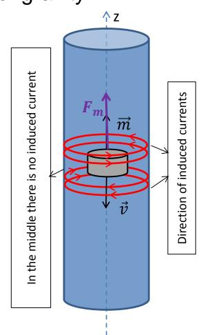
$\vec{m}$  – magnetic moment  $\vec{v}$  –velocity of a magnet
