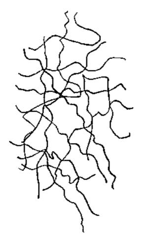
Rubber is composed of cross-linked polymer chains in constant movement
