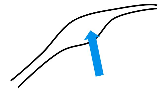
Thicker layer of rubber – stiffer, less strain
