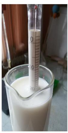
Example of calculation of milk density using a hydrometer.
