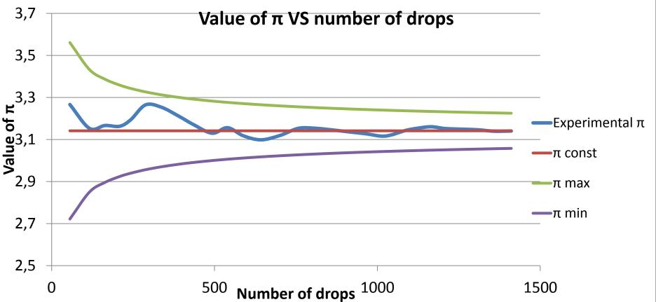
Conditions of experiment: Distance between the lines- 3 cmLength of the match- 4,2 cmFinal value of  $\pi$  - 3,1405405405
