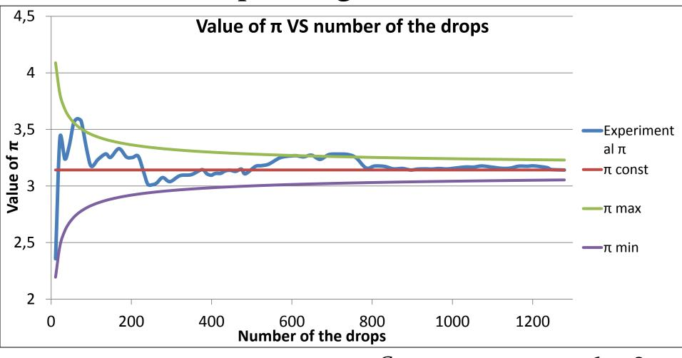
Conditions of experiment: Distance between the lines – 4,9 CM Length of the match – 4,2 CM Final value of  $\pi$ – 3,141219812 Constant  $\pi$  = 3,14159265358979 Difference between constant  $\pi$ and experimental  $\pi$ : 0,00037284
