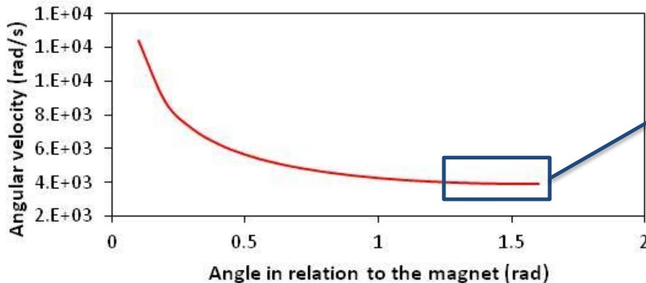
Angular velocity approximately constant near the normal line to the magnet.
