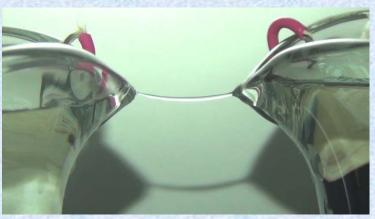
Weight of the bridge is  $Mg = \rho gAL_c$ . It is compensated by tension force  $Mg = 2\tau \sin \theta$
