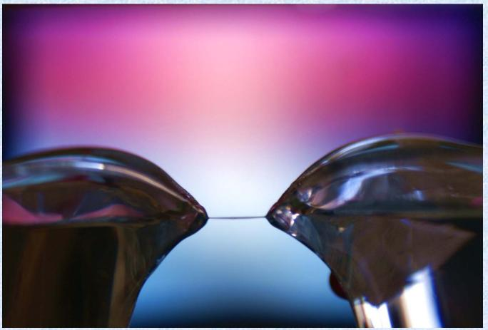
If a high voltage is applied to a fluid (e.g. deionized water) in two beakers, which are in contact, a fluid bridge may be formed. Investigate the phenomenon. (High voltages must only be used under appropriate supervision - check local rules.)
