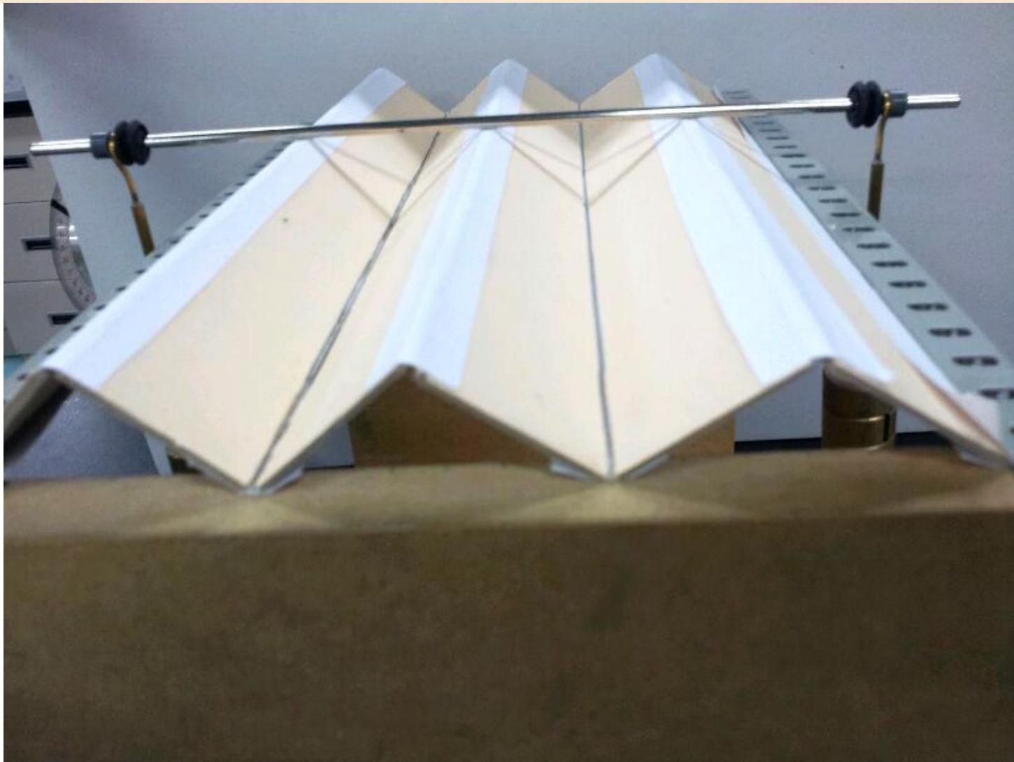
Thick paper bridge → eliminate necking and bending
