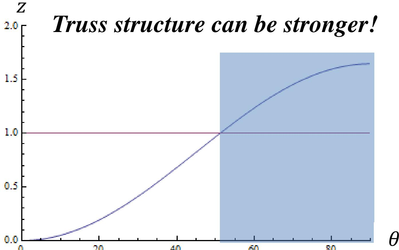
$$z = \frac{I_{z,truss}}{I_{z,tube}} = \frac{\pi^2(1 - \cos 2\theta)}{12}$$
