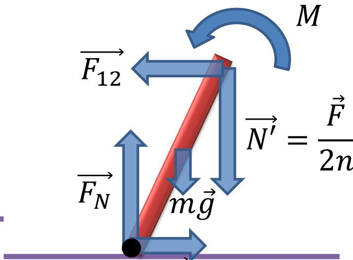
$$\begin{aligned} M &= -EI \frac{d^2w}{dx^2} = N'l \cos \theta + \frac{mgl \cos \theta}{2} - F_{12}l \sin \theta \\ &= \frac{1}{n^2} \left( \frac{FD}{4} \cos \theta + \frac{MgD \cos \theta}{8} \right) - \frac{fD}{2n} \sin \theta \end{aligned}$$
