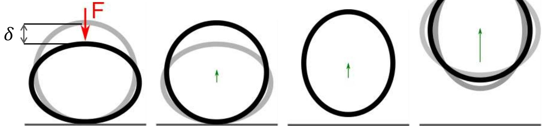
$$E_{BENDING} = \oint_{PERIMETER} \frac{IY}{2R_{CUR}^2} dl$$
