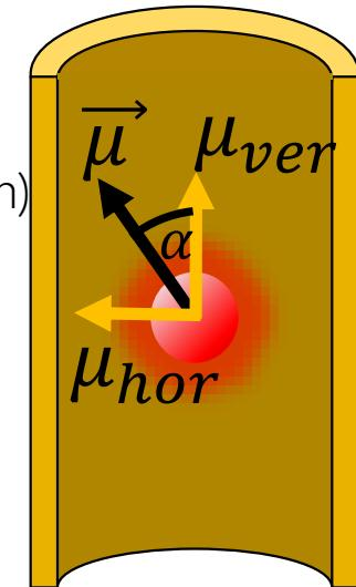
Associated radial fields (Flowing perpendicular to tube)
