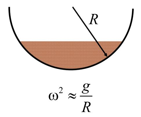
Resonant frequency weakly depends on the depth until the depth becomes comparable with the radius
